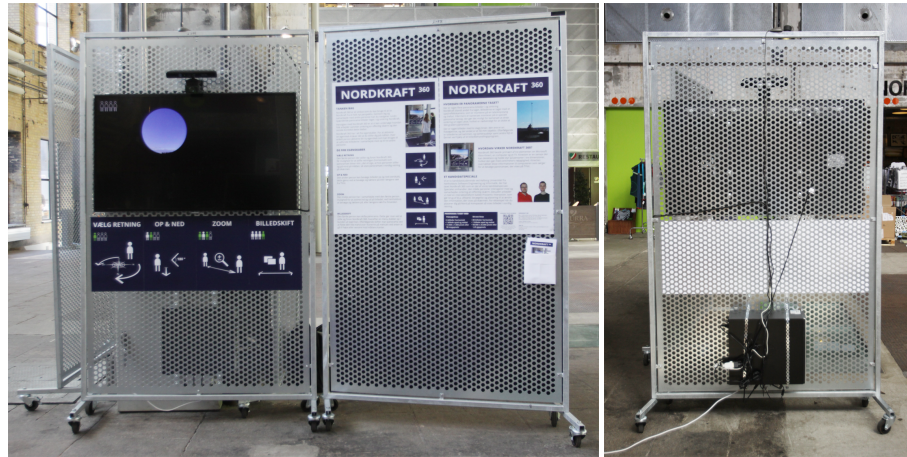
Fig. 1. To the left an image of Nordkraft 360, showing the four interaction illustrations beneath the display, along with the interaction and information poster hanging to the right of the system. To the right the back of the system is shown, with the computer and cables attached to the metal stand.
